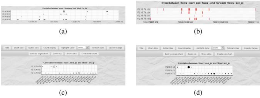
Fig. 2. Scatterplot and Gantt chart: (a) a scatterplot of connection counts over time by destination IP; (b) a Gantt chart of time ranges for flows by source IP; (c) a scatterplot with frequency count mapped to the size of an \times glyph; (d) a scatterplot with count mapped to circle size
