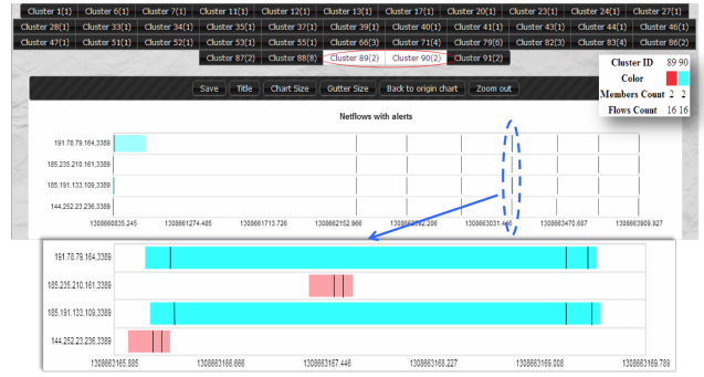
Fig. 7: Visualization of four flow ensemble members from two different clusters shown in blue and red
