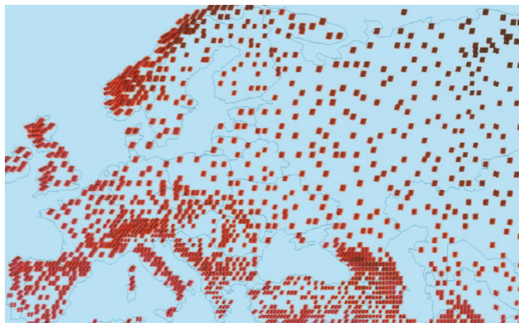
2 Multidimensional weather data over Europe and Asia reduced with our feature-preserving simplification system. In this example we are applying Hoppe's quadric mesh simplification algorithm. Color represents temperature (blue for cold to red for hot), size represents pressure (larger for higher), and orientation represents precipitation (vertical for light to horizontal for heavy). Dense glyph regions show areas with rapid spatial variation in attribute or terrain values, sparse regions show areas of slow variation.
