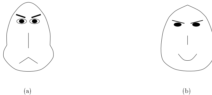
Figure 2.14: Examples of Chernoff faces: the various facial characteristics, such as nose length, eyes, mouth, jowls, etc., are controlled by various data values in each face
