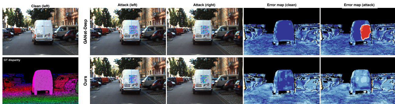
Figure 1. Examples of attacking stereo matching in the KITTI2015 [29] dataset. GANet-Deep [48] results on the top row, our results on the bottom row. The attack is based on the proposed stereo-constrained projected gradient descent (PGD) attack within a patch, which by design preserves the photometric consistency of non-occluded regions. One of the state-of-the-art methods, GANet-Deep shows a significant drop in performance (the last column), while the proposed method shows much stronger resistance to the attack.
